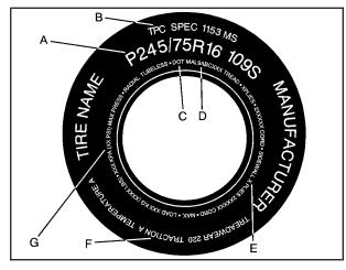
(A) Tire Size: The tire size code is a combination of letters and numbers used to define a particular tire's width, height, aspect ratio, construction type, and service description. See the Tire Size illustration later in this section for more detail.
